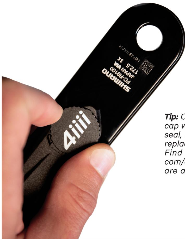
**Tip:** Check the condition of the o-ring on the battery cap when replacing your battery. To ensure a watertight seal, keep the o-ring lubricated with silicone grease and replace any o-rings that appear worn or damaged. Find the PRECISION Maintenance Tutorial video at [4iiii.com/docs](http://4iiii.com/docs). Replacement battery covers and o-rings are available from our online store.
