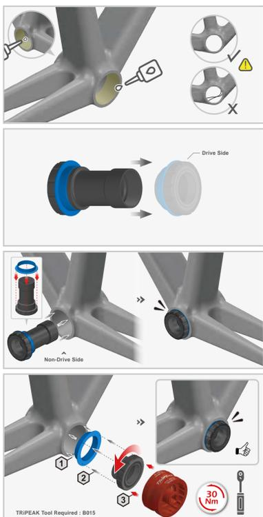
**Installation of Crank's Adapter**
